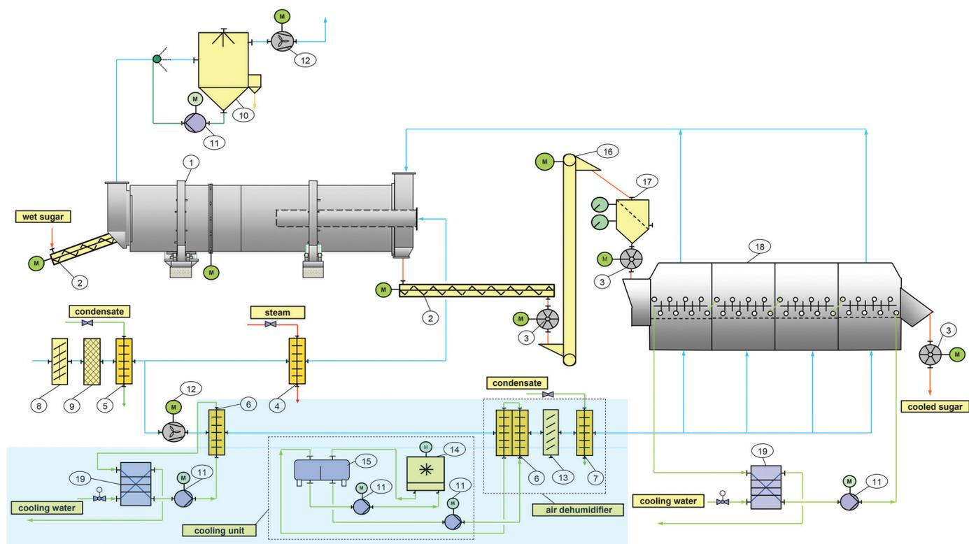
Fig. 2: Option 2 – Drum dryer with horizontal fluidised-bed cooler (caption please see Fig. 3)
