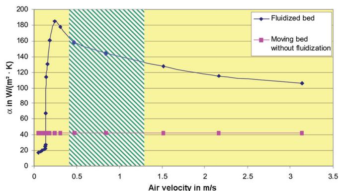
**Fig. 5:** Heat transfer rate in fluidised-bed coolers between heat transfer surface and product
