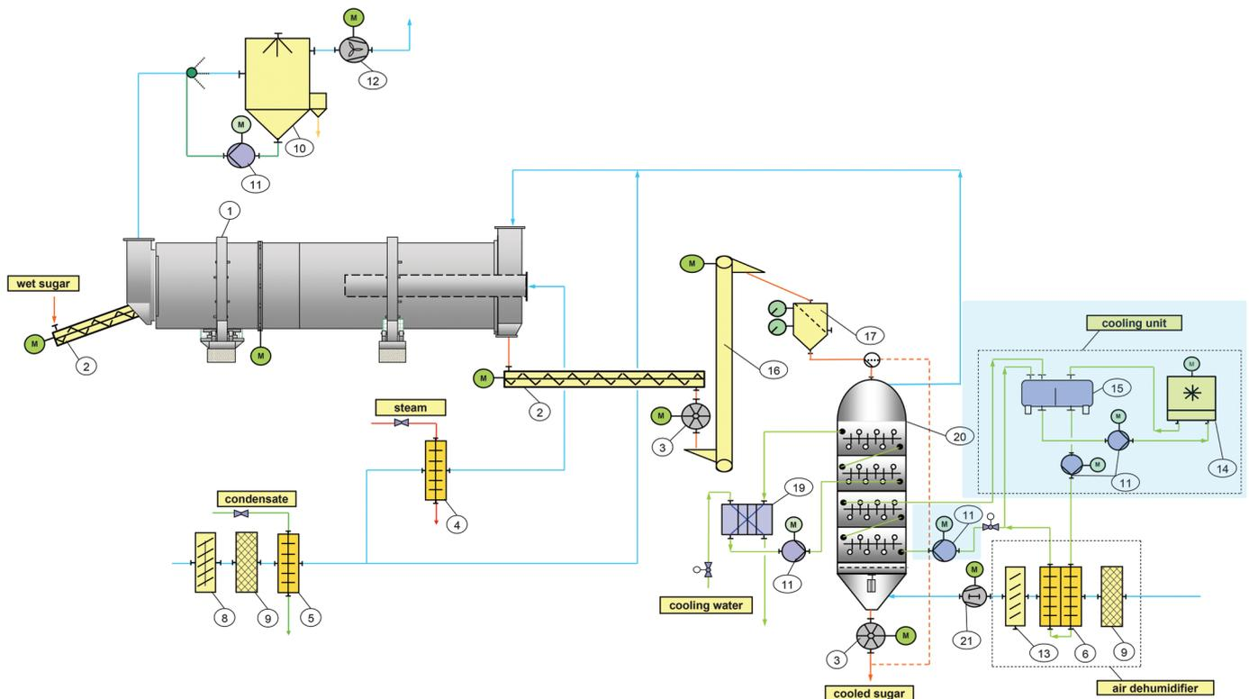
**Fig. 3:** Option 3 – Drum dryer with vertical fluidised-bed cooler & air conditioner
